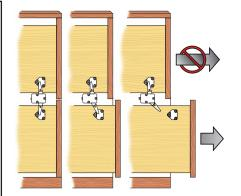
WHEN EITHER DRAWER IS PULLED OPEN, THE DRAWER CLIP ON THAT DRAWER MOVES THE SNAPPER INTO A LOCKED POSITION. THIS PREVENTS ANY FURTHER DRAWERS FROM BEING OPENED.
