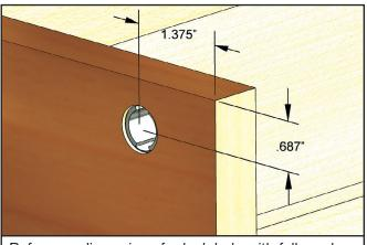
Reference dimensions for lock hole with full overlay drawer and 3/4" end panel.
