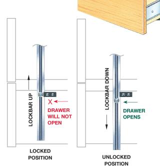
When used with the AP-037 3/8" Adjustable Pin, a strong, rigid lock is provided.
